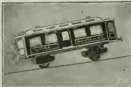
Up She Goes—the Real Gyro-Monofleter Imported from Toyland. The Metal Car Measures 9 1/2 Inches Long, 4 Inches High, and 2 1/4 Inches in Width. The Small Revolving Gyroscope That Stabilizes It, as It Rolls Along a Cable or Single Track, Is But 2 1/2 In Diameter. Fitted With Propellers, Such a Car Ascended an Inclined Cable in the Same Manner as Proposed and Described in the August Issue.
