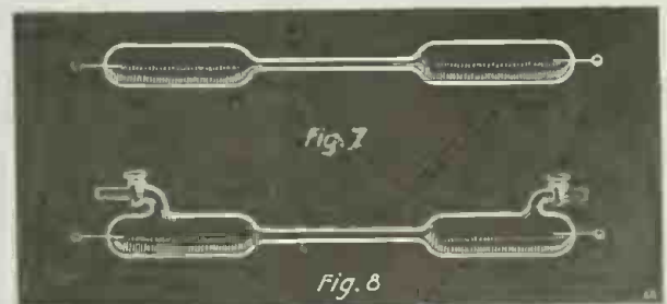
Sealed and Experimental Forms of Glass Tubes in Which Gas is Placed. The Wires Are Connected to a Spark Coil and the Glowing Tube Examined Before the Spectroscope.
