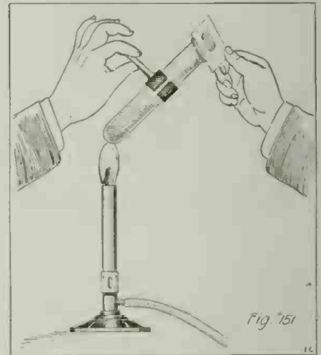
Applying the Lead Acetate Test to Hydrogen Sulfid Gas.
